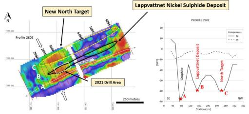
Slingram survey results. Strongest conductors are in red. Western half of the survey employed a 60-metre coil configuration and a 40-metre coil configuration was used for eastern part of the survey block. The larger discordant red anomaly in the easternmost part of the survey is likely resulting from conductive soils.
