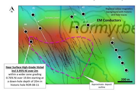
In addition to prioritizing these EM targets outside the current resource for drilling, the Company plans to evaluate potential for higher-grade nickel shoots within the Rormyrberget deposit.
