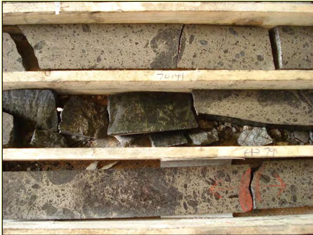
Figure 7-4: Mineralized Intersection from the Lappvattnet Deposit. LAP07-002: 3.21%Ni, 0.06%Cu, 0.08% Co over 4.97m (76.43-81.40m)
